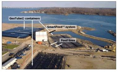
mately 2,000 linear feet of pipeline conveyed dredged effluent from the work area to the SmartFeed<sup>™</sup> system.
